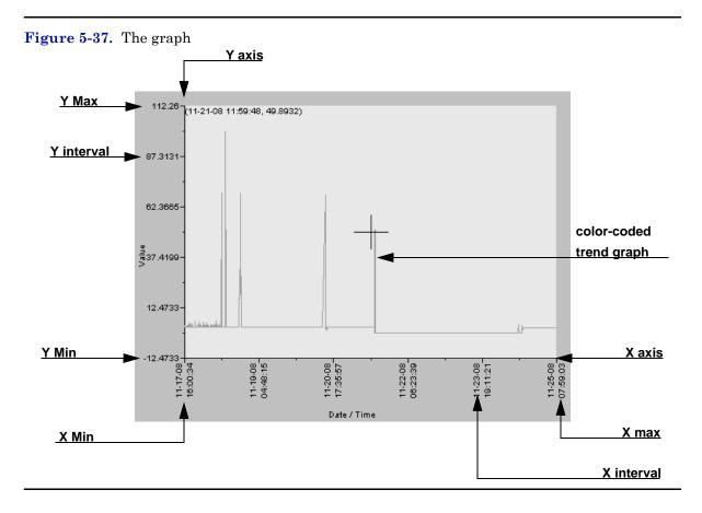
Click **Edit** to view or change the display properties of the X and Y axes. The *Edit Graph* window displays.
